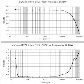
divtube ST70 driver closed loop 35W output
