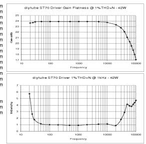
diytube ST70 driver closed loop 1%THD at 1kHz • 1.165Vrms input
