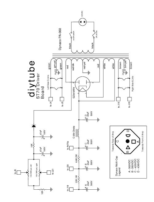
Note: This diagram shows the original twist-lock can capacitor. If you have the SDS Labs capacitor board or other power supply upgrade, please refer to documentation for your board or upgrade.
