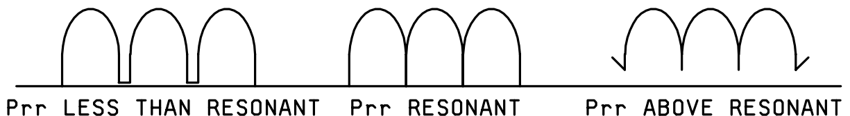
FIGURE 5. Charging current waveforms with charging diode .
